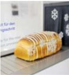
Nitrogen, e.g. for the Crust-freezing of white bread to ensure better slicing
