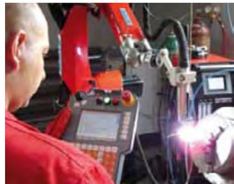
Plasma-powder surfacing is a computer-controlled process.
