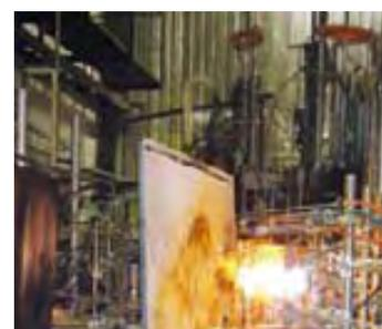
Liquid oxygen is used for flame polishing.
