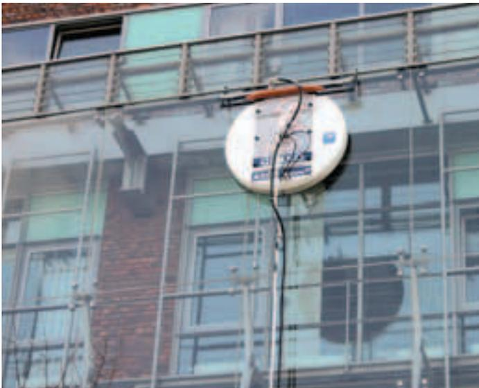
*The Gekko® cleans glass facades in an environmentally friendly way using dry ice.*
