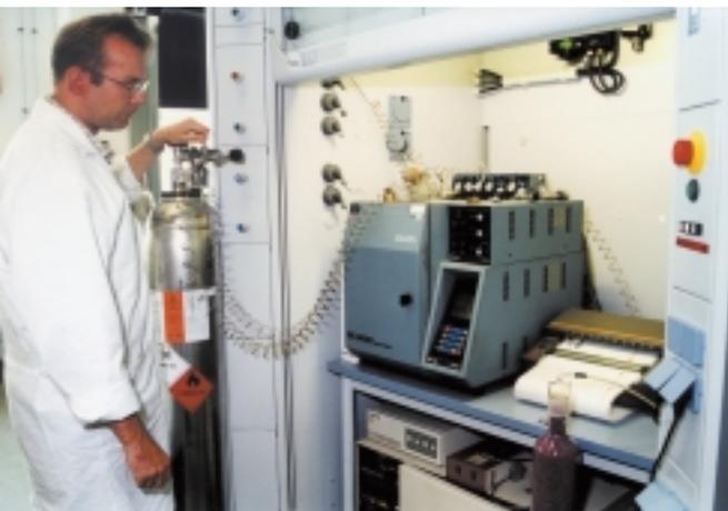
Calibration gas test on the gas chromatograph at the special gases plant in Krefeld-Gellep
